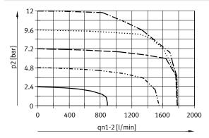
Flow direction 2 > 3; as a function of output pressure p2
