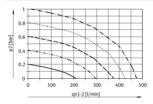
Flow rate qn for valves with pressure regulation range 0 ... 2 bar Flow direction 1 > 2; as a function of output pressure p2
