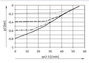
Flow rate qn for valves with pressure regulation range  $-1 \dots +1$  bar Flow direction 1 > 2; as a function of output pressure p2
