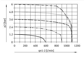
Flow rate qn for valves with pressure regulation range 0 ... 10 bar Flow direction 1 > 2; as a function of output pressure p2
