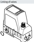
Up to five valves can be linked using connecting kit VAME-P18-K-P5. The connecting kit consists of two square nuts, two socket head screws and an O-ring.
