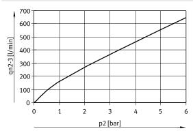
Flow direction 2 > 3; as a function of output pressure p2
