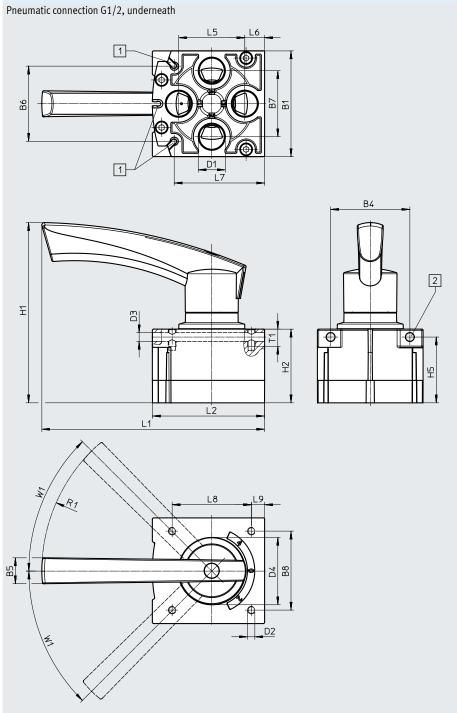
[1] Slot for proximity switch [2] Mounting hole SM...-10...
