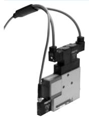
This vacuum generator has an identical design to the other VADMI types. This ejector also has an integrated vacuum switch with air saving function: If the pressure drops below the set vacuum range, vacuum generation is switched on automatically.
