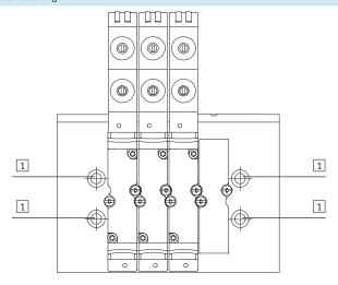
The CPA-SC valve terminal is screwed onto the mounting surface using four M4 screws.
