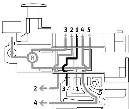
The reversible B regulator splits the supply air in duct 4 and regulates the pressure upstream of the valve in duct 3 (the unregulated pressure from duct 1 is in duct 5). The regulated air is then supplied to duct 2. The valve is thus operated in reversible mode.
