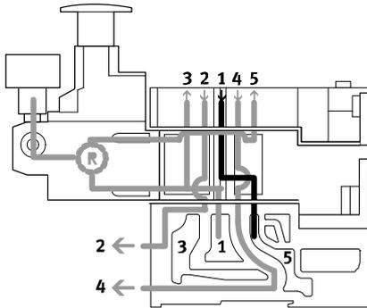
The reversible A regulator splits the working air in duct 1 and supplies the pressure upstream of the valve into duct 5 (the unregulated pressure from duct 1 is in duct 3). The regulated air is then supplied to duct 4. The valve is thus operated in reversible mode.
