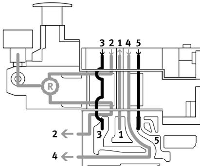
This pressure regulator regulates the pressure in duct 2 after the pressure medium flows through the valve. During venting, the exhaust flow in the valve is from duct 2 to duct 3 via the pressure regulator.
