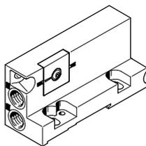
For end plates with selector switch, the outgoing direction of the ports is to the front of the valve terminal. This means that all of the ports on the terminal can be combined in one outgoing direction. A special feature of the right-hand end plate is the selector switch that
