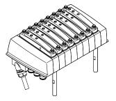
The signals are transmitted from the controller to the valve terminal via a pre-assembled or self-assembled multi-wire cable to the multi-pin plug connection. This substantially reduces installation time. The valve terminal can be equipped with max. 32 solenoid coils. This corresponds to 2 to 32 valves. The multi-pin cable should be no longer than 30 m.
