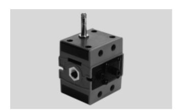
Solenoid actuated soft start valve for gradual pressure build-up in pneumatic systems. This ensures safe start-up of pneumatic systems. A minimal amount of air flows into the system via an adjustable flow control valve. Output pressure is built up slowly. Downstream cylinders and working devices are slowly advanced to their initial positions. When the
