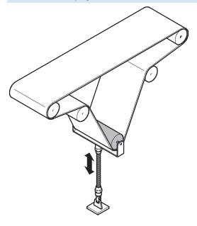
In dusty or dirty environments, a hermetically sealed fluidic muscle has a major advantage over conventional drives. This seal cannot wear. It is a sturdy, contractible tube that copes with the tough demands of the cement industry with ease.
