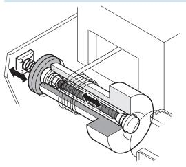
The friction-free muscle allows uniform and gentle braking of the pay-out reel, ensuring highly precise winding at constant speed. Control is provided by a proportional control valve whose signals are regulated via force sensors.
