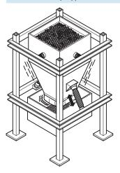
Hoppers and silos are susceptible to the problem of parts jamming during feeding. Fluidic Muscle facilitates stepless regulation of a pneumatic shaker between 10 and 90 Hz, thereby guaranteeing continuous delivery.
