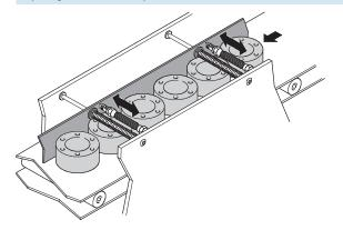
With small batch sizes, it is often necessary to adapt entire system sections to different component dimensions after a short period of time. This task can be performed with the fluidic muscle in cases where an approximate adjustment is sufficient.
