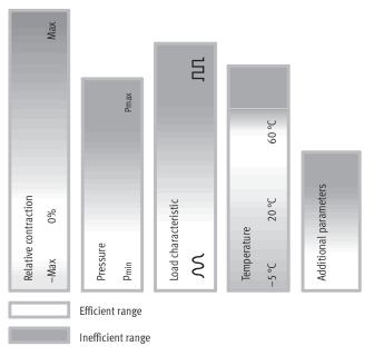
The service life of the fluidic muscle is between 100000 and 10 million switching cycles for typical applications. Optimisations can be made using the information from the left diagram. The service life thus increases due to a reduction in the
