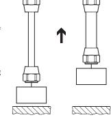
Fluidic Muscle behaves like a spring with a changing external force: it follows the direction of action of the force. With Fluidic Muscle, both the pretensioning force of this "pneumatic spring" and its spring stiffness can be varied. Fluidic Muscle can be
