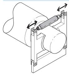
The fluidic muscle is setting new standards in applications that require fast response times. The emergency stop for rollers demands both speed and force. Long machine downtimes in the event of malfunctions can thus be prevented.
