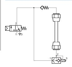
The service life of the Fluidic Muscle depends on the contraction, the operating pressure and the temperature. High operating frequencies or high loads can lead to a temperature rise. Targeted pressurisation on one side
