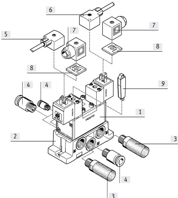
Solenoid valve with central plug M12, 3-pin
