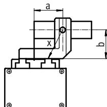
The gripping force  $F_h$  can then be read from the graphs (→ page 6) using the calculated value x.
