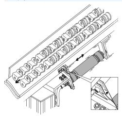
The Fluidic Muscle is exceptionally well suited to transporting or aligning parts. Amplitude and cycle rate can be adjusted simply and independently of each other. The muscle's flexibility makes it possible to set the optimum conveying speed for any conveying process.
