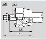
MAS-...-EA/BA – pneumatic connection, axial, one end/both ends
