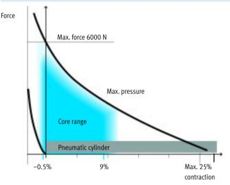
The muscle expands lengthways when it is pretensioned by an external force. When pressurised, on the other hand, the muscle contracts, i.e. its length decreases.
