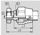
MAS-...-ER/BR – pneumatic connection, radial, one end/both ends
