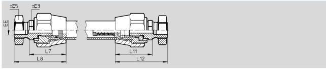
MAS-...-ER/BR – pneumatic connection, radial, one end/both ends
