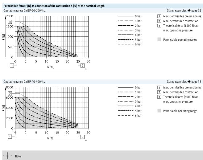
The actual value of the force as a factor of the contraction can vary according to the product characteristics and the ambient conditions present.
