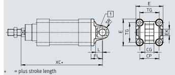
[1] The pivot pin is secured against rotation with a spring pin.
