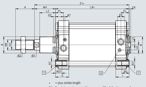
[1] Special outer hex nut with female thread for mounting components [2] Adjusting screw for adjustable end-position cushioning (PPV)
