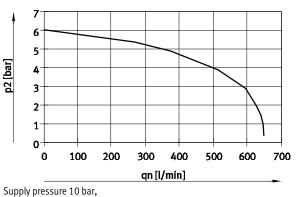
Supply pressure 10 bar, set regulator pressure 6 bar
