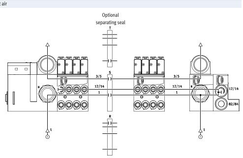
External pilot air supply, ducted exhaust air
