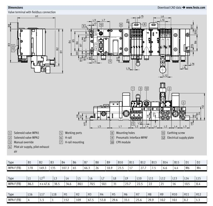
1) n = number of sub-bases (with MPA1, width 10 mm, max. 4 valve positions on sub-base; with MPA2, width 20 mm, max. 2 valve positions on sub-base)
