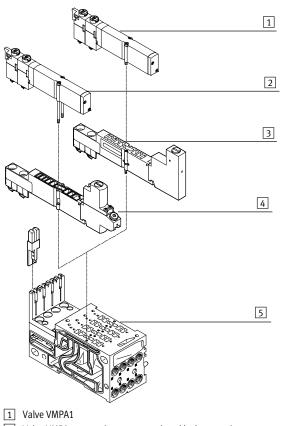
Vertical stacking components, MPA2
