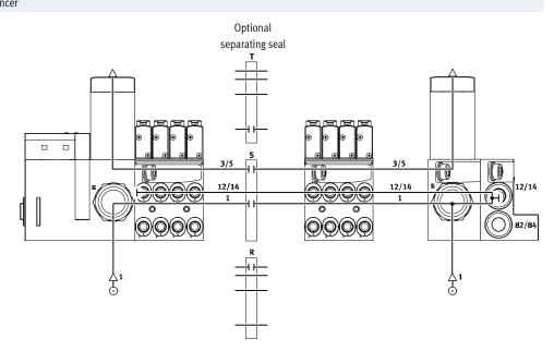
External pilot air supply, flat plate silencer
