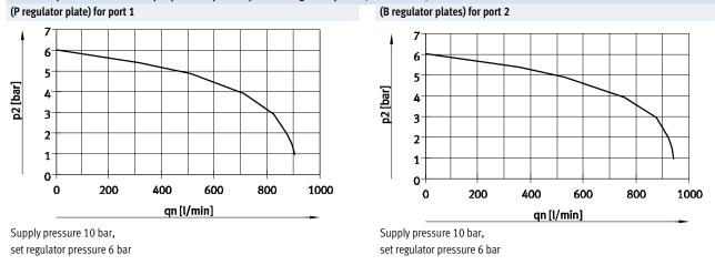
Flow rate qn as a function of output pressure p2 with pressure regulator plates (width 20 mm) (A regulator plates) for ports 4 (B regulator p
