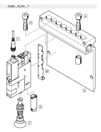
1) Hollow bolt 9 and mounting bracket 10 are included in the scope of delivery of the OVEM-...-PL/PO-....
