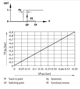
The switching point is determined from the teach-in point and the functional reserve. A functional reserve (35% of the teach-in pressure) is subtracted from the teach-in pressure (SP = TP - 0.35\*TP). For example, a switching point of -0.33 bar is set at a teach-in pressure of -0.5 bar. The hysteresis is fixed.
