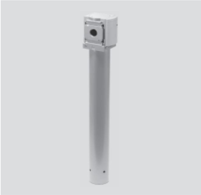
Membrane air dryers remove water vapor from the compressed air and lower the dew point preventing moisture from forming downstream. Pre-filtration with a grade of 0.01 micron is required.
