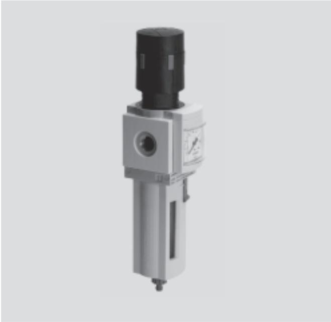
A filter regulator combines a filter and a pressure regulator into a single unit. The sintered filter with water separator removes contamination, pipe sinter, rust and condensate from the compressed air. The pressure setting can be adjusted with the regulator.
