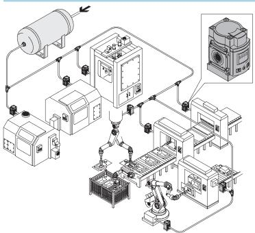
• Compressed air consumption and function monitoring of various systems in the production process
