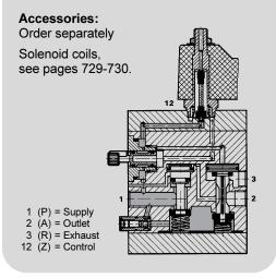
Festo "Soft-start" valves are designed to provide slow pressure build-up in pneumatic systems preventing sudden high pressure air surges during start-up. Manual override is built in.
