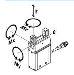
The indicated permissible forces and torques apply to a single gripper jaw. They include the lever arm, additional applied loads due to the workpiece or external gripper fingers and acceleration forces occurring during movement.
