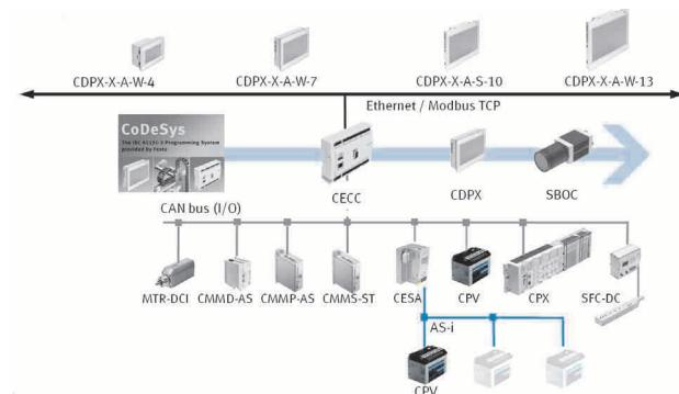
The CECC can communicate with all electric drive controllers from Festo and actuate all valve terminals via CANopen.
