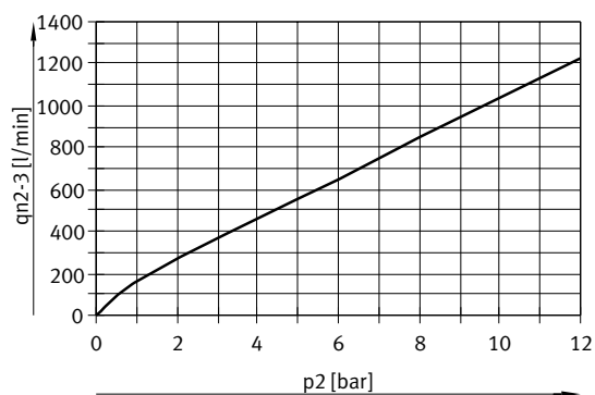
Flow rate q_n from 2 > 3 as a function of output pressure p_2
