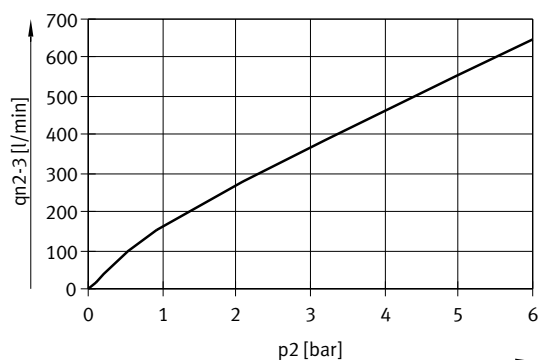
Flow rate q_n from 2 > 3 as a function of output pressure p_2
