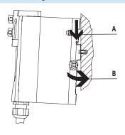
The VTSA-F valve terminal is hooked onto the H-rail (see arrow A).
