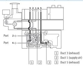
This pressure regulator regulates the pressure upstream of the valve in duct 1. Ducts 2 and 4 thus have the same regulated pressure.
