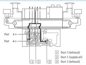
With this pressure regulator, the supply air (duct 1) is split and routed directly to both pressure regulators. In each case the regulated supply air is present in ducts 3 and 5 on the valve. The valve is thus operated in reversible mode.
