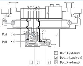
This pressure regulator regulates the pressure in ducts 2 and 4 after the pressure medium flows through the valve. During venting, the exhaust flow in the valve is from duct 2 to duct 3 and from duct 4 to duct 5 via the pressure regulator.
