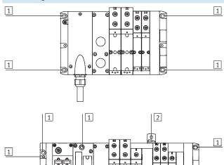
The VTSA-F valve terminal is screwed onto the mounting surface using M6 screws. The mounting holes are located at the following points:
