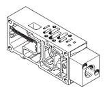
Modified manifold sub-bases (width 42 mm) are available for the soft-start valve. This manifold sub-base supplies the pressure zone on the valve terminal with compressed air and provides a high flow range. The pneumatic interface to ISO5599-1 is
