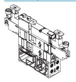
Additional functions can be added to each valve position between the manifold sub-base and the valve. These functions are known as vertical stacking modules, and enable special functioning or control of an individual valve position. Combinations of several valve sizes on one valve terminal are possible.
