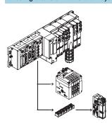
The optional string extension enables additional valve terminals and I/O modules to be connected to the fieldbus node of the CPX terminal. Different input and output modules as well as CPV-SC, CPV and CPA valve terminals can be connected. The maximum length of the CP string
