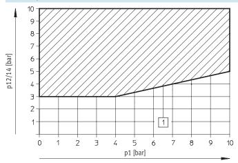
1 Operating range for valves with external pilot air supply
