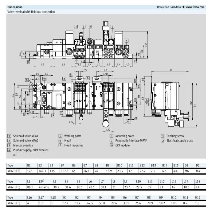
$<sup>1) \</sup>quad \text{n=number of sub-bases (with MPA1, width 10 mm, max. 4 valve positions on sub-base; with MPA2, width 20 mm, max. 2 valve positions on sub-base)} \\$
