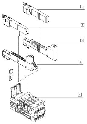
Vertical stacking components, MPA2
