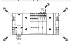
The MPA-F valve terminal is screwed onto the mounting surface using four M6 screws. The mounting holes are on the pneumatic interface and on the right-hand end plate.
