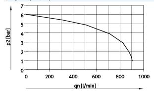
Supply pressure 10 bar, set regulator pressure 6 bar
