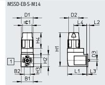
[1] Insert can be repositioned by 90°
