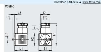
[1] Insert can be repositioned by 90°
