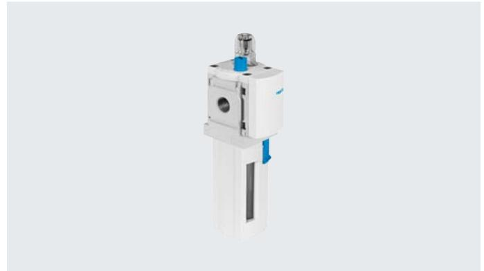
The proportional lubricator adds a precisely adjustable amount of oil to the compressed air. The pressure drop that occurs when air flows through a Venturi nozzle is used to feed oil from the container to the drip cap.
