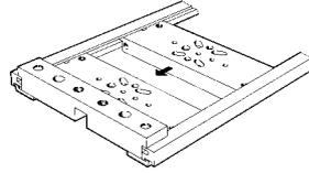
They can also be placed onto the frame and screwed down individually.
