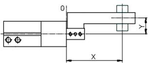
Gripping forces at 6 bar as a function of eccentric application of force (distance from the zero co-ordinate line
