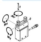
The indicated permissible forces and torques apply to a single gripper jaw. They include the lever arm, additional applied loads due to the workpiece or external gripper fingers and acceleration forces occurring during movement.
