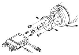
If feature EHPS-...-RA1 is used, the delivery includes all the connection components in addition to the gripper:
