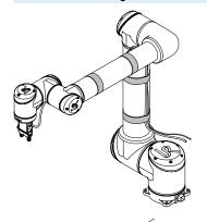
The gripper with robot connection EHPS-...-RA1 enables fast integration on a light-weight robot.
