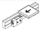
Example Given: Friction coefficient  $\mu = 0.1$ Conveying speed v = 12 m/min Conveyed goods m with workpiece carrier = 25 kg
