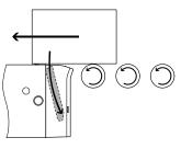
Position 3 Stopper cylinder is in the release position The stop is retracted and the conveyed item is released LED status message: open Input signal: 1
