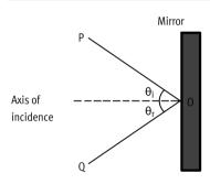
Specular reflection is the perfect reflection of light (or other kinds of wave) from a surface, when incident light from a single direction is reflected in a single direction
