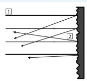
Diffuse reflection is the reflection of light from an uneven or grained surface when an incident beam is reflected at many different angles.
