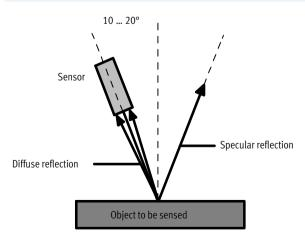
In the case of diffuse sensors with intensity differentiation, diffuse sensors with background suppression and distance and colour sensors, sensing is based on diffuse reflection. These sensors therefore require as much diffuse reflection as possible. Total reflection makes detection difficult and must therefore be avoided
