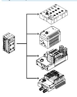
The CPX-CTEL master provides 4 external I-Port interfaces, each of which can be connected with a device. I-Port is an interface for exchanging serial data for connecting decentralised modules or valve terminals from Festo. The I-Port interface is based on IO-Link and is compatible with it in certain areas. The connection type corresponds to a star topology. In other words, only one module or valve terminal can be connected to each I-Port. The restrictions compared to IO-Link include:
