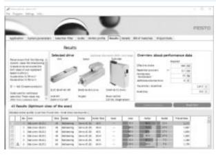
Create the optimum drive package quickly and reliably. PositioningDrives calculates suitable combinations of electric axis, electric motor and servo drive from just a few application details. You sort the results according to your specifications and obtain all the relevant data including the bill of materials and documentation for the selected combination. This avoids design errors and results in significantly improved energy efficiency for the system.
