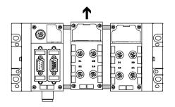
The mechanical connection between the CPX modules is established using special tie rods. Two screws in the end plates are all that are needed to mount the entire unit. The tie rod ensures that the unit resists high mechanical loads and is therefore the "mechanical backbone" of the CPX terminal.
