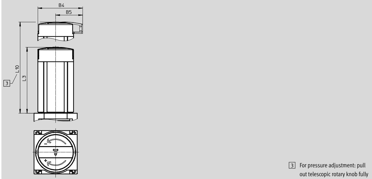
[3] For pressure adjustment: pull out telescopic rotary knob fully
