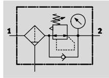
Fully automatic condensate drain, with pressure gauge
