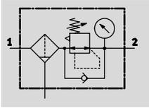
Manual rotary condensate drain,
