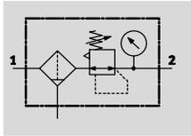
Semi or fully automatic condensate drain, with pressure gauge
