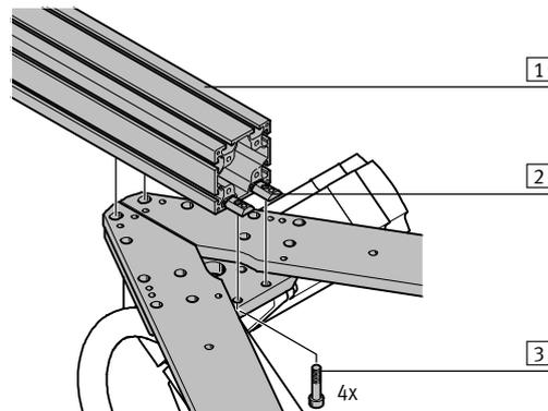
Mounting via slot nuts – at right angles to the mounting frame
