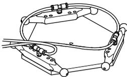
The rod loss detection feature detects detached rods and initiates an emergency stop.
