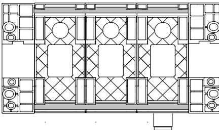
The mechanical connection between the CPX modules is established using special tie rods. Two screws in the end plates are all that are needed to mount the entire unit.
