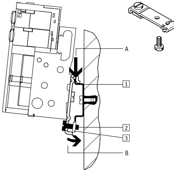
The valve terminal is attached to the H-rail (see arrow A) and then swivelled on the H-rail and secured in place with the clamping component (see arrow B).
