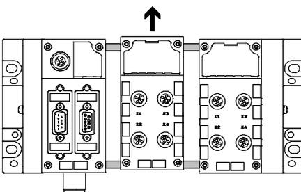
The open design allows interlinking blocks to be replaced in the assembled state.
