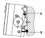
The MPA-L valve terminal is attached to the H-rail (see arrow A). The terminal is then swivelled onto the H-rail and secured in place with the clamping component (see arrow B).
