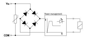
Each solenoid coil is protected with a spark arresting protective circuit as well as against polarity reversal. All valve types are additionally equipped with integrated current reduction.
