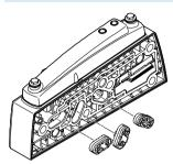
If different working pressure levels are required, the MPA-C offers a range of options for creating pressure zones. Duct 1 and/or duct 3 and/or duct 5 are blocked by inserting a separator in the sub-base. Each pressure zone must have its own supply. The following supply options are available:
