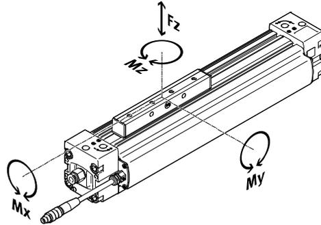
If the drive is simultaneously subjected to several of the forces and torques listed below, the following equation must be satisfied in addition to the indicated maximum loads:
