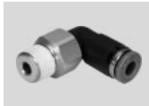
Push-in fitting with swivel connection, rotatable by 360°. The ball bearing enables rotating movements in the application up to max. 500 rpm. For pneumatic applications with a temperature range up to 60 °C and a pressure range up to 14 bar.
