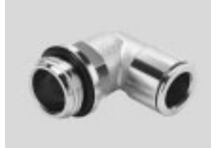
Attractively priced metal push-in fitting for pneumatic applications with a temperature range up to 70 °C and a pressure range up to 16 bar. Tubing O.D.∅ of 3, 4, 6, 8, 10, 12 and 14 mm with connecting threads M5, M7 and G $\frac{1}{8}$  ... G $\frac{1}{2}$ .
