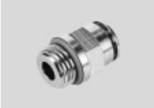
All metal push-in fitting made of chemically nickel-plated brass. High corrosion resistance (CRC3) and chemical resistance. For pneumatic applications with a temperature range up to 150 °C and a pressure range up to 20 bar.
