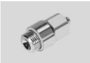
Stainless steel fitting for use in areas subject to intensive cleaning. Highest level of corrosion resistance (CRC 4). For pneumatic applications with a temperature range up to 120 °C and a pressure range up to 12 bar.
