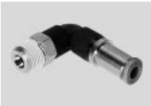
Push-in fitting that blocks the air flow after the tubing is disconnected. For pneumatic applications with a temperature range up to 60 °C and a pressure range up to 14 bar.
