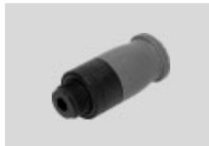
Plastic fitting for easy installation with one-hand operation. Hydrolysis resistant, FDA compliant and easy to clean. For pneumatic applications with a temperature range up to 60 °C and a pressure range up to 10 bar. Tubing O.D. 6 mm with connecting thread G $\frac{1}{8}$ .
