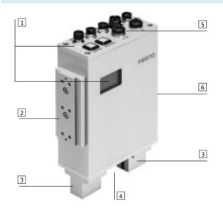
The Checkbox Compact CHB-C-N provides 24 V DC high-power signals at its outputs, which can be used to directly actuate quick-switching pneumatic valves, for example the MHE2-MS1H-, without using external interface assemblies or controllers, in order to reliably filter faulty or incorrectly oriented parts out of the parts flow using an air jet. Other types of actuators such as pneumatic or electrical ejectors, deflectors or turning stations can also be controlled.
