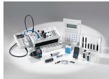
PLCs and I/O Devices PLC's, operator interfaces, sensors and I/O devices
