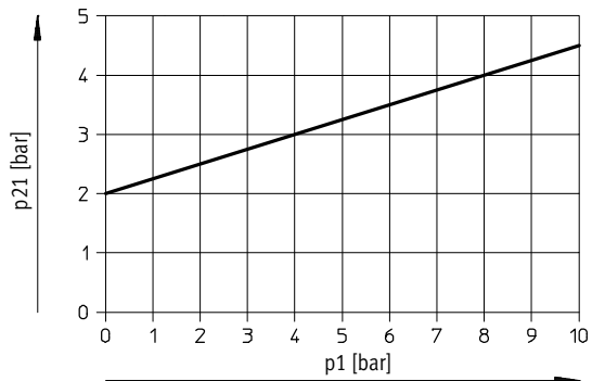
Minimum pilot pressure p_{21} as a function of operating pressure p_1
