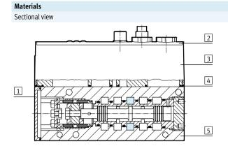
Proportional directional control valve 1 Cover Reinforced polyamide Inscription panel 2 Polyester 3 Electronics housing Reinforced polyamide 4 Seals Nitrile rubber 5 Valve housing Anodised wrought aluminium alloy Note on materials RoHS-compliant
