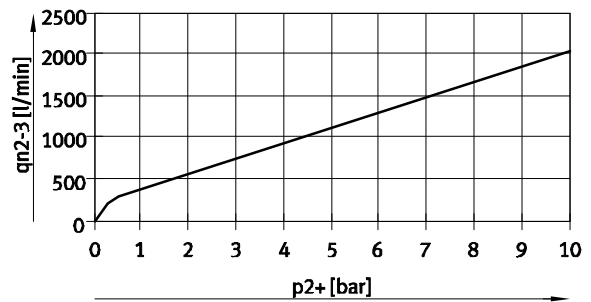
Flow rate q_n from 2 \rightarrow 3 as a function of output pressure p_2
