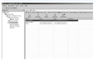
Recording can be started once the camera has been set up. You can choose whether the camera should wait for the occurrence of an external trigger condition, start recording directly following initialisation or store the pictures sent via Ethernet on a PC without buffering them in the camera. The PC can be removed once recording has been started in "Wait for trigger
