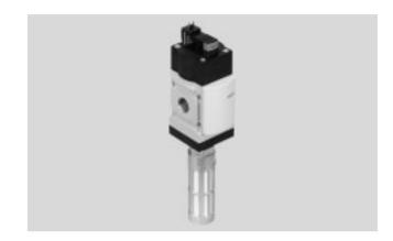
Electro-pneumatic soft-start and quick exhaust valve for gradual pressurisation and quick exhausting of system components (single channel). The main flow control valve in the cover permits a gradual build-up of output pressure p2. Once the output pressure p2 has reached the set pressure switchover point (switching pressure), the valve opens and the full operating pressure p1 is present at the output.
