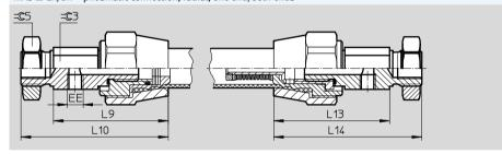
$MAS-...-EA/BA-EG/BG-pneumatic connection, \ radial, \ with \ threaded \ rod, \ one \ end/both \ ends$
