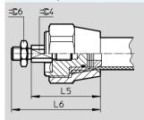
MAS-...-EA/BA – pneumatic connection, axial, one end/both ends
