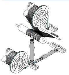
The spring properties of the Fluidic Muscle make it exceptionally well suited to regulating the thread tension when winding threads. The tension in the threads is always as high as it needs to be for the process in question. This means that the optimum thread tension is always available, leading to better protection of the threads and counteracting wear on all components.
