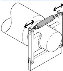
The Fluidic Muscle is setting benchmarks in applications that require fast response times. The emergency stop for rollers demands both speed and a high initial force. This can prevent risks to the operator in the event of malfunctions.
