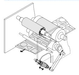
The Fluidic Muscle is exceptionally well suited to pressing on rollers. The contact pressure can be varied using the operating pressure. The design means that components do not become stuck and there are thus no peak forces. The Fluidic Muscle is hermetically sealed and can be disconnected from the compressed air supply. It will nevertheless continue to perform its function.
