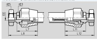
MAS-...-ER/BR – pneumatic connection, radial, one end/both ends
