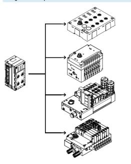
The CPX-CTEL master provides 4 external I-Port interfaces, to each of which a device can be connected. I-Port is an interface for exchanging of serial data for connecting decentralised modules or valve terminals from Festo. The I-Port interface is based on IO-Link and is compatible with it in certain areas.
